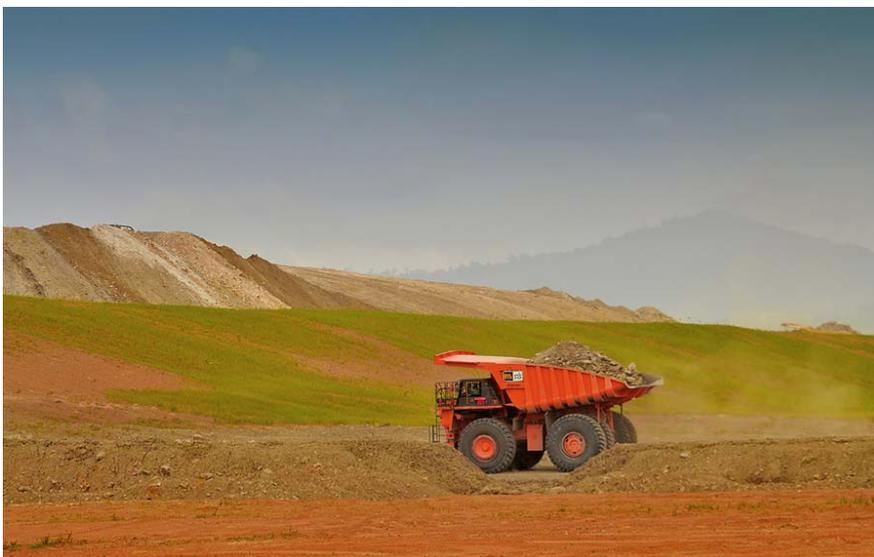
*One of SIS's dump truck hauls 150 tonnes of overburden to the overburden dumping area which is located 4-6 km away from the pit*
