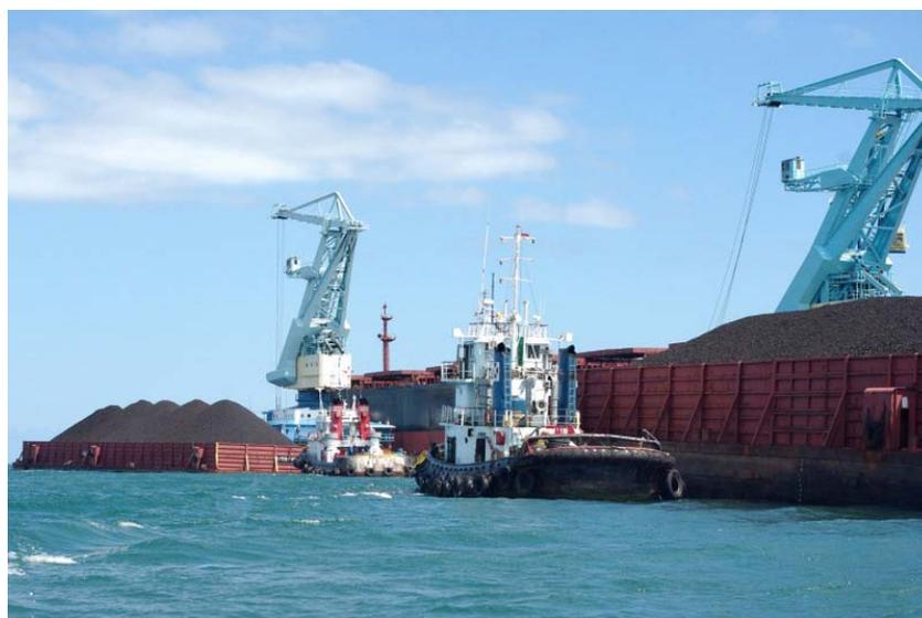
*Loading the coal from Adaro's barges to an 80,000 tonne Panamax vessels using MBP's floating cranes*
