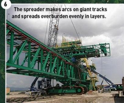
6 The spreader makes arcs on giant tracks and spreads overburden evenly in layers.
