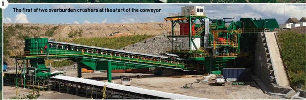
1 The first of two overburden crushers at the start of the conveyor
